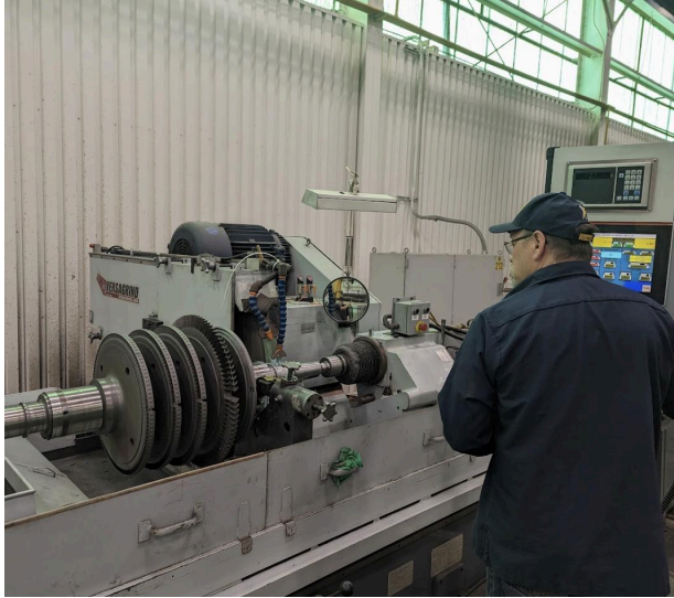
Precision cylindrical grinding of a turbine rotor can achieve OEM dimensional tolerances and surface finish.
