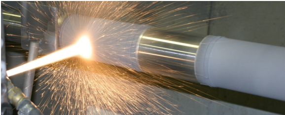
HVOF thermal spray applied to a rotating shaft at HFW.
