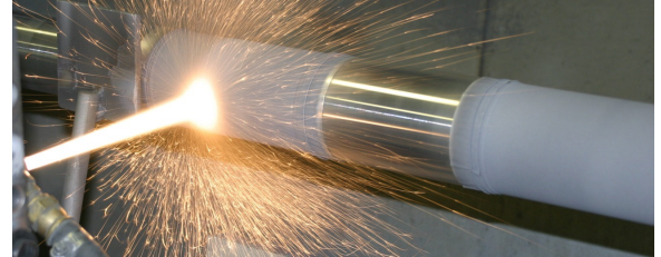
HVOF thermal spray applied to a rotating shaft at HFW.
